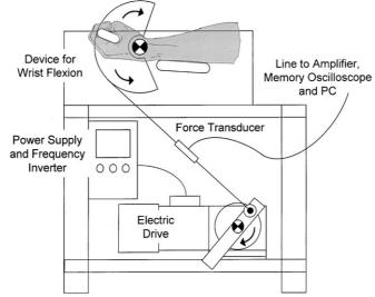
Fig. 2. Isokinetic movement apparatus (a, b) existing of a frame where the electric drive (5), power supply (4) and one of the three movement devices (1) is mounted. A flexible steel cable with a piezoelectric force transducer (3) is connected to the drive (6) allowing an almost sinusoidal reciprocating motion in the movement device. Real time measurement is performed by means of an oscilloscope and a PC (2).
