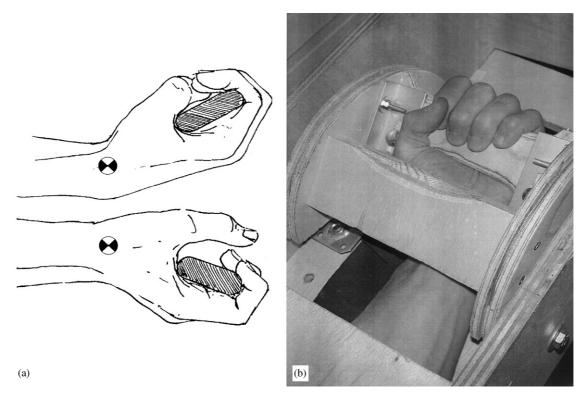
Fig. 3. Wrist flexion device (b) allowed eccentric and concentric flexion of the wrist of  $30^{\circ}$  on each side (a) of the neutral position (extension and flexion).
