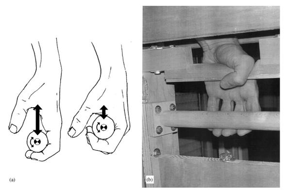
Fig. 4. Device for "rolling in and out a bar" movement (b) allowed eccentric and movement with all fingers (except the thumb) with a range of motion of the interphalangeal joints not more than  $40^{\circ}$ . The free turning bar was mounted on a gliding sled. An anatomically shaped handle, which was grasped by the thumb and thenar acted as a resistance against the flexion movement. Linear range of motion of the bar was 40 mm (a).
